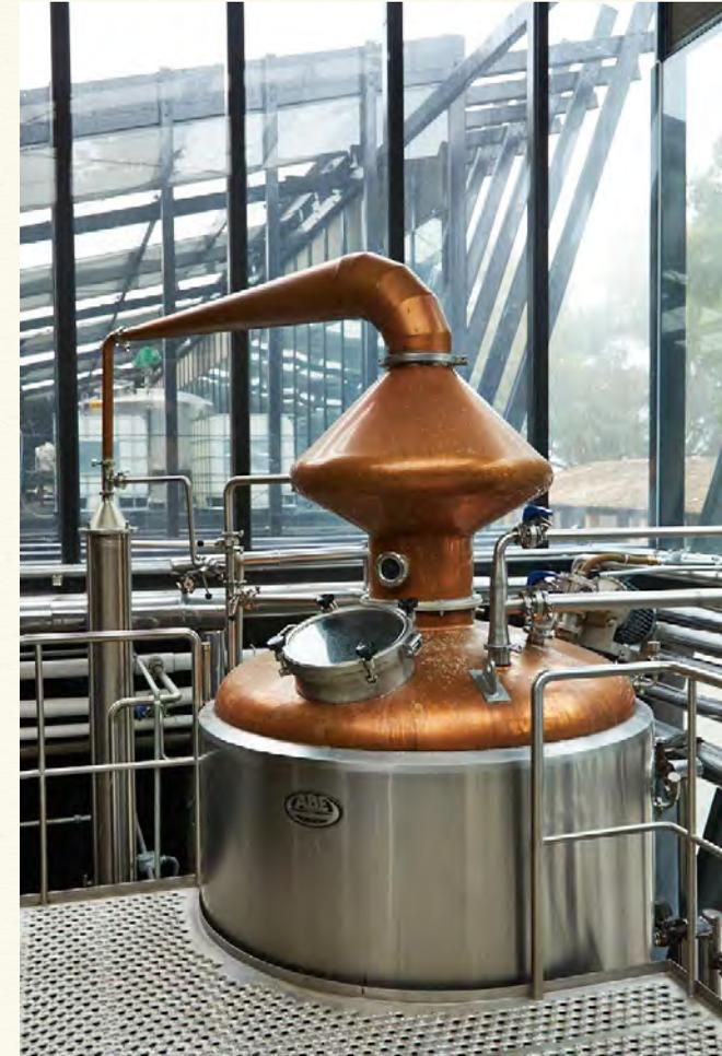
Fermented wort is poured into traditional copper stills to make a first distillation where the volatile compounds are trapped, creating a wonderful spirit that emerges at 40% ABV. A second and slow distillation concentrates the alcohol at 62.5% ABV making it ready for aging.
